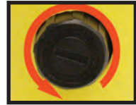
Turn knob counter clockwise to decrease pressure.
