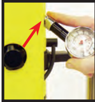
Pressure gauge on Schrader Valve.
