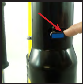
A. Turn on/off valve to the off position, by pushing down on the switch.
