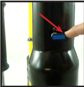
A. Turn on/off valve to the off position, by pushing down on the switch.
